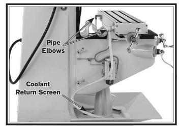
Figure 13. Coolant return hose connections.
